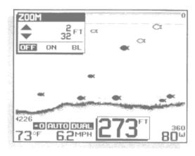
Another form of range control is Zoom. Zoom allows selection of various ranges for full screen viewing, while maintaining a view of the full range. By using the display to view a smaller area, the effective display resolution is increased, and the units ability to separate targets close together is enhanced.
